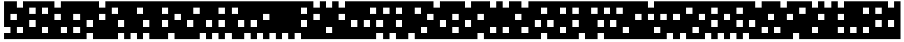
Figure 3. The binary pattern used in the structured light modules for sewer inspection features a uniqueness window size of 6 \times 6 and a minimum Hamming distance of 3. This pattern is concatenated both horizontally and vertically to fill the entire projector image.
