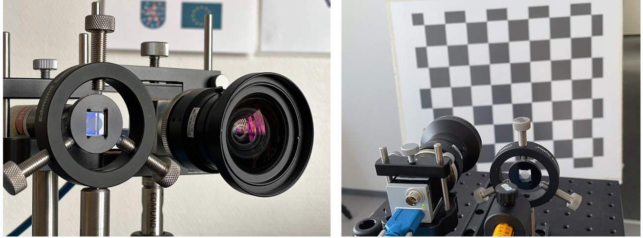
Figure 6. An experimental setup featuring a 2.35 MPix camera, collimated laser, and DOE. The setup was geometrically calibrated using a checkerboard target, visible in the background on the right.
