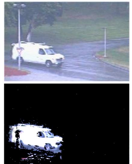
Figs. 8 and 9: Initial image and results of object detection with the multiple Gauss procedure, during strong rainfall
