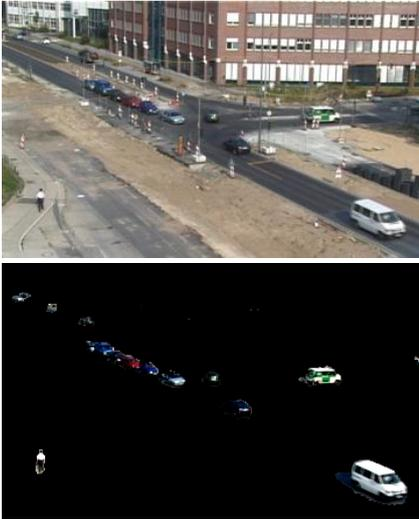
Figs. 4 and 5: Multiple Gauss procedure; source image and detection result
