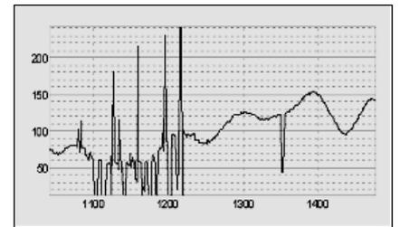
Fig. 3: Intensity over time of an image pixel in the roadway area of a traffic scene, size of the image series: 500 images (5 images/s), intensity spikes: vehicles passing by
