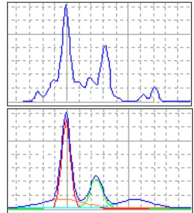
Figs. 6 and 7: Histogram over time and multiple Gauss approximation of a single pixel
