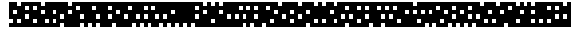
Figure 3: Binary pattern with uniqueness within a window size of 6 \times 6 which is used in the structured light modules. The pattern is repeated horizontally and vertically to fill the entire projector image.
