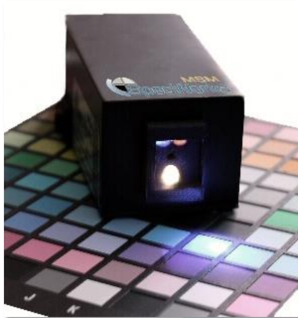
SpecWorks™-MSM-VIS prototype for spectral incident light measurements
