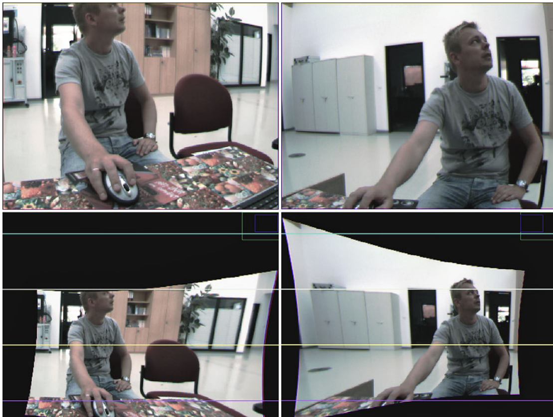
Fig. 6.5: Result of image rectification and rectification with drawn epipolar lines (below) of the input images (above).
